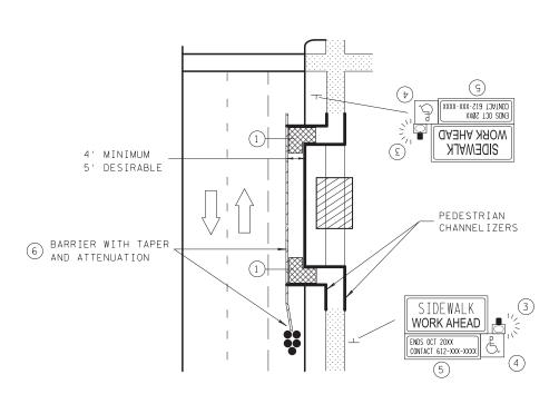
SIDEWALK BYPASS USING SHOULDER OR PARKING LANE HIGH SPEED ROADWAY
